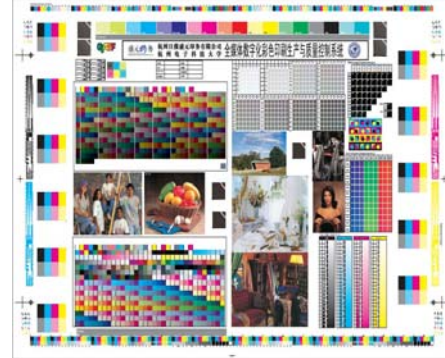
Figure 3 Self-correcting output color patch of Konica Minolta C6000 digital press
